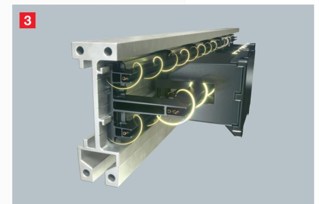
➔ And what's more – with MOVITRANS®, the power socket rides along, as it were. Energy is transferred without contact via an air gap, allowing for an electromagnetic connection that is completely wear-free and maintenance-free. This contactless energy supply also makes it possible to achieve high speeds.
