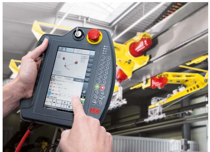
RobotMonitor can be run on both a PC and a separate control plate, meaning you always have the same user interface available for operation. The movement can be conveniently defined using SRL (the "SEW Robot Language" interpreter language) and teach-in mode.
