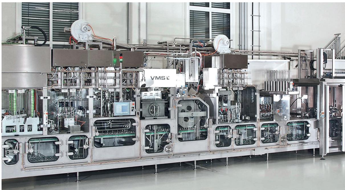
**Aseptic food filling:** Sophisticated motion control topologies promote flexible modularity in systems, as demonstrated by this example of a cup-filling machine with the highest hygiene requirements.
