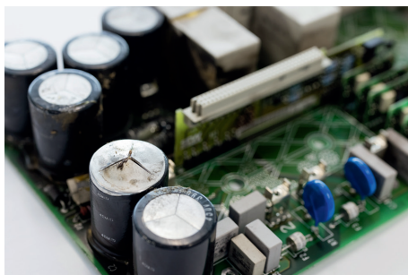
Forming to prevent capacitor explosions
