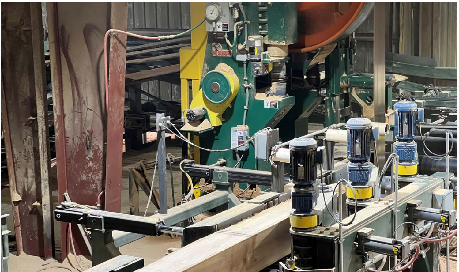
The addition of electromechanical synchronized electric cylinders and synchronized integral motor reducers ensure increased precision for less waste.
